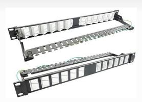
The flat 1U 24-port panel is design to accept keystone jack seated in angles inside the panel and result the connected patch cables automatically run to the cabinet/rack side to eliminate additional routing to horizontal cable manager/panel to save consumption of rack space. Flat design is ideal for installation within telecom cabinet as well as rack.
